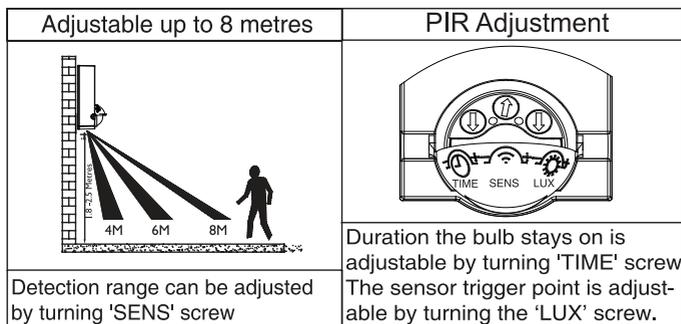
To access the adjustment screws, flip down the black cover over the PIR sensor.
