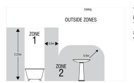
This product has no special protection against the ingress of moisture, and is rated as IP20.
