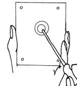
7. Feed supply cable from house supply through hole in soft grommet which will form a seal around the cable
