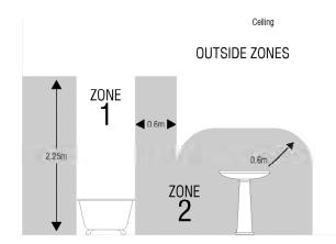
This product is suitable for use in Zone 2 and outside Zones of a bathroom. See diagram. If this unit is being fitted in a room containing a bath or shower, a 30mA RCD must be used, in accordance with IEE regulations.
