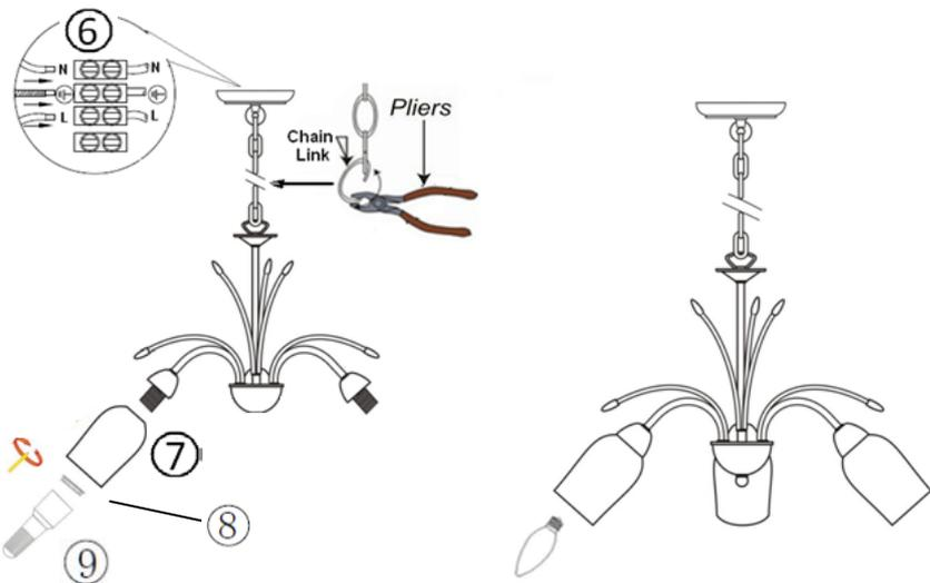
Details of terminal wiring.
