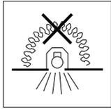
Ensure free movement of air around the fitting by removing any roof void insulation from at least 140mm around the hole.
