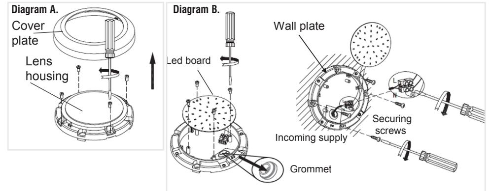
4 retaining screws on the sides of the unit. Unscrew these to remove the lens housing.
