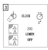
After mode 2, press the switch to change to mode 3. Product will be 290Lm when motion is detected and will turn off after 25 seconds.
