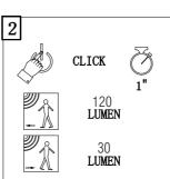
After mode 1, press the switch to change to mode 2. Product will stay on at 30Lm and increase to 120Lm when motion is detected (This will stay at 120Lm for 25 seconds then dim to 30Lm and stay lit).
