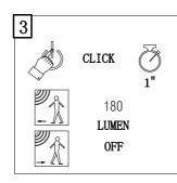
After mode 2, press the switch to change to mode 3. Product will be 180Lm when motion is detected and will turn off after 25 seconds.
