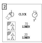
After mode 1, press the switch to change to mode 2. Product will stay on at 20Lm and increase to 70Lm when motion is detected (This will stay at 70Lm for 25 seconds then dim to 20Lm and stay lit).
