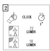
After mode 1, press the switch to change to mode 2. Product will stay on at 18Lm and increase to 72Lm when motion is detected (This will stay at 72Lm for 25 seconds then dim to 18Lm and stay lit).
