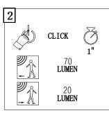
After mode 1, press the switch to change to mode 2. Product will stay on at 20Lm and increase to 70Lm when motion is detected (This will stay at 70Lm for 25 seconds then dim to 20Lm and stay lit).
