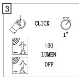
After mode 2, press the switch to change to mode 3. Product will be 180Lm when motion is detected and will turn off after 25 seconds.
