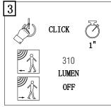
After mode 2, press the switch to change to mode 3. Product will be 310lm when motion is detected and will turn off after 25 seconds.
