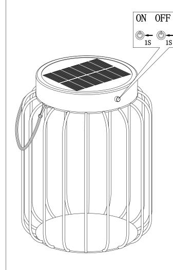
NOTE - This product will only illuminate at dusk. It will not be able to be operated during daylight.
